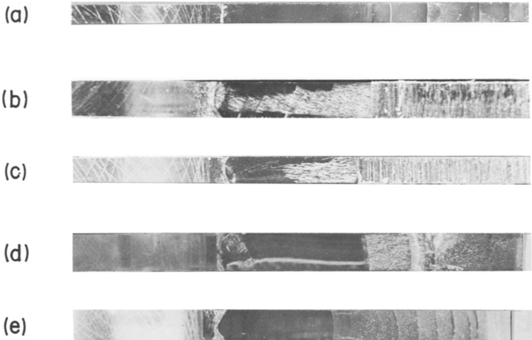
Figure 2 Fracture surfaces of (a) poly(vinyl chloride), (b) polycarbonate, (c) polysulphone, (d) polystyrene and (e) poly(methylmethacrylate).
